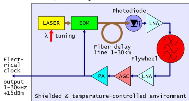
Figure 14: Electro-optical master oscillator.
