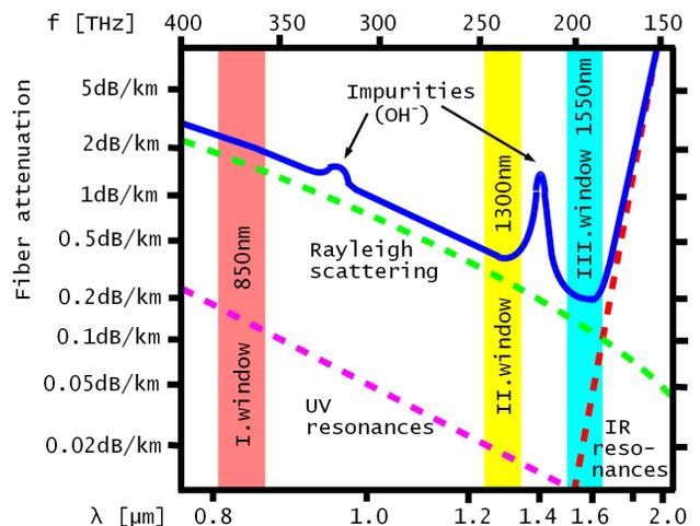
Figure 4: Silica-glass fiber attenuation.
