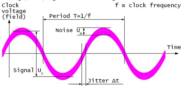
Figure 1: Signal-to-noise ratio & timing jitter.
