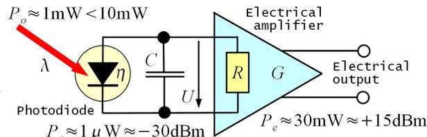
Figure 7: Photo-diode receiver.
