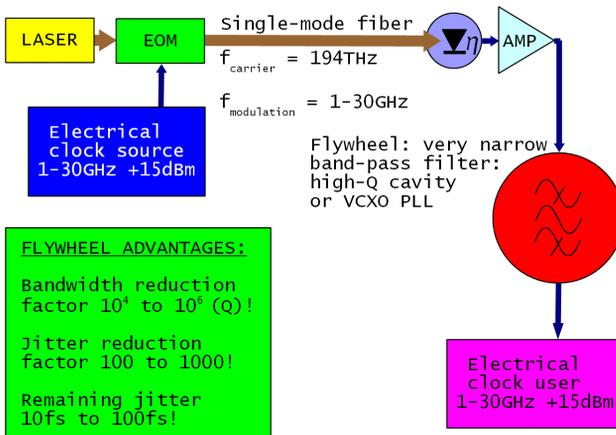
Figure 8: CW modulation system with flywheel.
