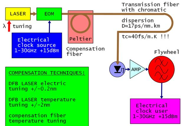
Figure 9: Delay-variation compensation techniques.
