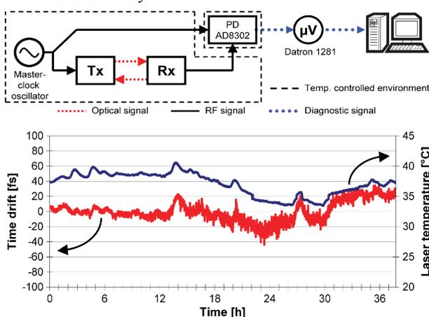
Figure 12: Measured long-term drift at 3GHz.
