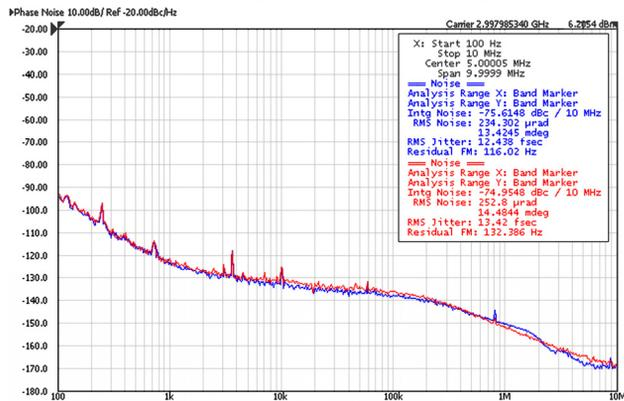
Figure 11: Measured phase noise & jitter at 3GHz.
