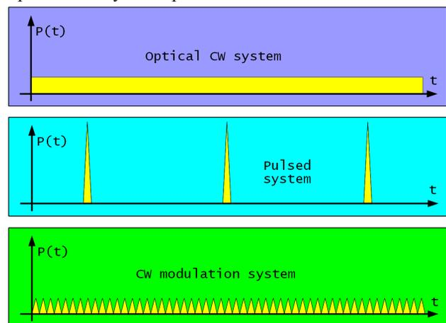
Figure 6: Optical timing systems.
