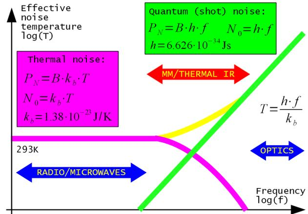
Figure 2: Thermal and quantum noise.
