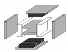
Figure 4: Recycler permanent magnet gradient dipole components shown in an exploded view. For every 4" wide brick there is a 0.5" interval of temperature compensator material composed of 10 strips.
