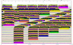
Figure 8: Mountain range plot showing 11 batch slip stacking process. Horizontal scale is 10 µsec.
