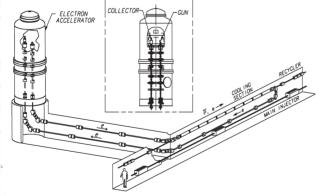
Figure 7: Schematic layout of the Recycler electron cooling system and accelerator cross section (inset) [22].
