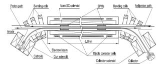
Figure 10: General layout of the Tevatron Electron Lens.
