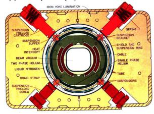
Figure 3: Cross-section of the Tevatron SC dipole magnet.
