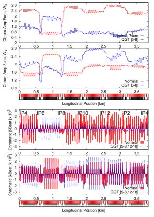
Figure 6: Chromatic W-functions for the nominal lattice at  $\beta^* = 0.7$ m and lattice with  $\gamma$ -T quadrupoles used to minimize them in the IR6 and IR8 regions.
