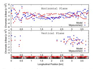
Figure 3: Chromatic  $\beta$ -beating in the Blue ring with gold ions at 100 GeV and 0.7m  $\beta^*$ .
