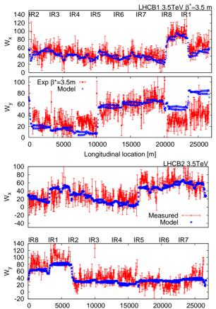
Figure 2: Chromatic W-functions for beam 1 and beam 2 in the LHC for 3.5 TeV at  $\beta^* = 3.5$  m
