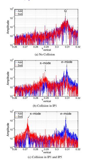
Figure 2: The Fourrier transform of the addition and subtraction of the beam position measured by the BBQ pick-ups.
