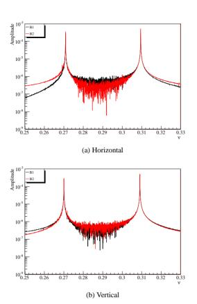
Figure 1: Simulation of coherent spectrum for the experiment 1. A tune shift of  $\Delta Q_{\rm sim} = 0.040$  is observed between the two coherent modes.
