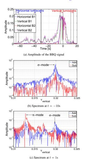
Figure 3: Amplitude of the BBQ signal during the instability and spectrum of the added and subtracted signals during the instability. t=0 is defined at the time of the observed emittance growth.
