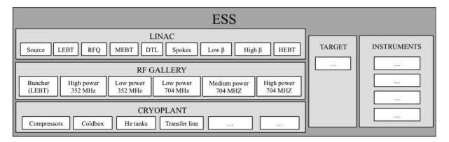
Figure 2: Schematic layout of the system structure.
