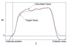
Figure 6: Designed magnetic field distribution and the target distribution (smooth curve).
