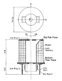
Figure 3: Permanent magnet for beam focusing in klystron at KEK (1987).
