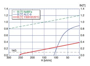
Figure 1: B-H curves of RE, ALNICO, and Ferrite magnets. RE magnets are strong but expensive. Historically well-known ALNICO magnets have high remanence but less coercivity. Anisotropic ferrite magnets have less remanence but stronger coercivity than ALNICO.
