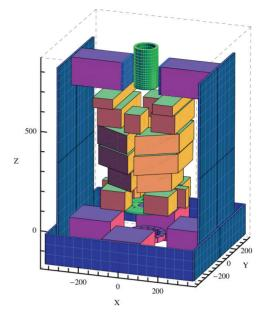
Figure 5: Permanent magnet focusing system designed with RADIA4.29
