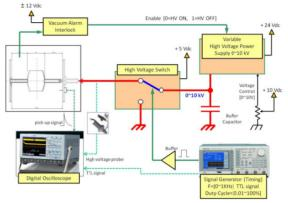
Figure 9: The chopper principle schematic test bench
