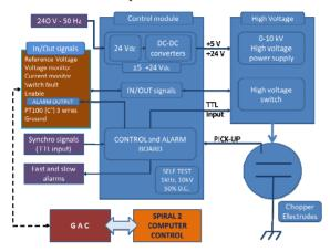
Figure 8: Block diagram of the slow chopper system.
