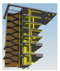
Figure 3: Architectural and structural models combined.
