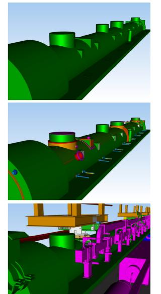
Figure 2: Accelerator module placeholder (top) with rf interface details (middle) and connected waveguides (bottom).
