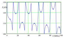
Figure 6: Estimation of Zc from the open/short method.
