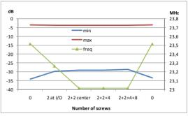
Figure 10: Sensitivity of the amplitude (dB) of the maximum and the minimum of the S<sub>11</sub> curve of Fig.4a and of the frequency (MHz) of the minimum.
