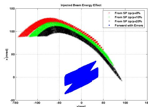
Figure 6: Phase space boundaries at the BEND1 entrance. Different errors of particle energy were assumed from 0%
