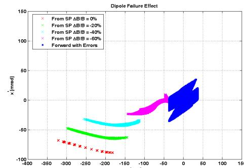
Figure 9: The phase space boundaries from the ID straight section and bending beamline begin to overlap once the strength of bending magnet BEND2 has fallen to 40% of its nominal value.
