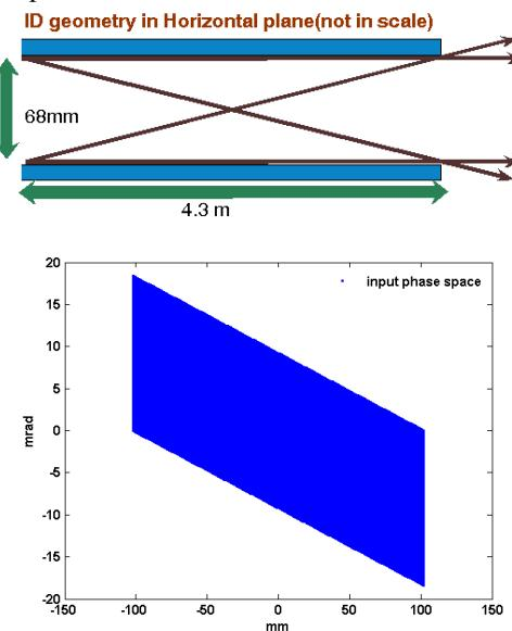
Figure 2: The input distribution used for forward tracking. The top figure indicates the possible motion of particle going through insertion device. The lower figure is the phase space for ID straight section.
