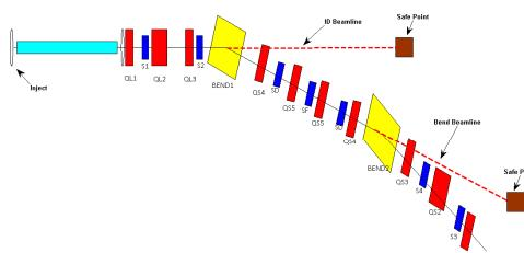
Figure 1: The locations of main accelerator components is shown in the layout of one unit section.
