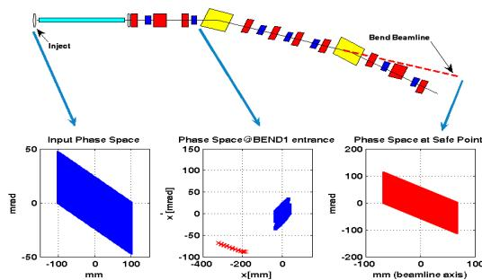
Figure 8: The top plot shows the bending beamline section of the storage ring. The lower left plot shows the initial phase space coordinates for the forward tracked beam. The lower right plot shows the initial coordinates for the backward tracked beam, and the lower middle plot compares the final two distributions.
