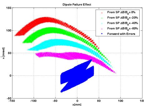
Fig 7: Phase space boundaries tracked to the BEND1 entrance for varying degrees of bending magnet failure.
