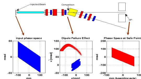
Figure 5: The top plot shows the ID beamline section in the storage ring. The lower left plot shows the initial phase space coordinates for the forwards track beam(blue), the lower right plot shows the initial coordinates for the back tracked beam(red), and the lower middle plot compares the final two distributions.
