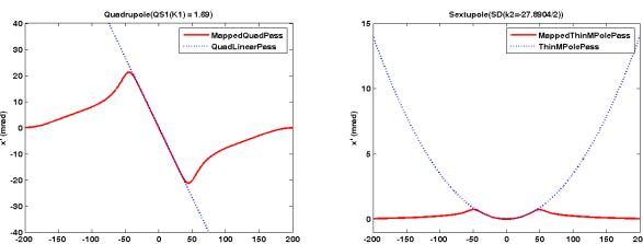
Figure 4: Results of particle tracking through a quadrupole (left) and a sextupole (right) using both new and old pass methods.
