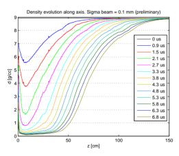
Figure 2: Density profiles along the longitudinal axis for 0.1mm sigma beam.
