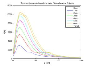
Figure 6: Temperature profile for 0.5mm sigma beam.
