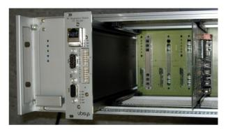
Figure 7 : RF Backplane and the M&D Module.
