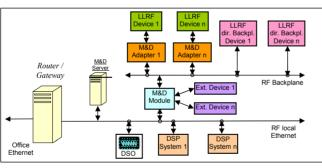
Figure 1 : Integration of different types of LLRF devices into the RF backplane standard.
