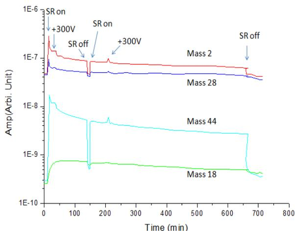
Figure 7: Real-time mass spectrum for an OFHC absorber
