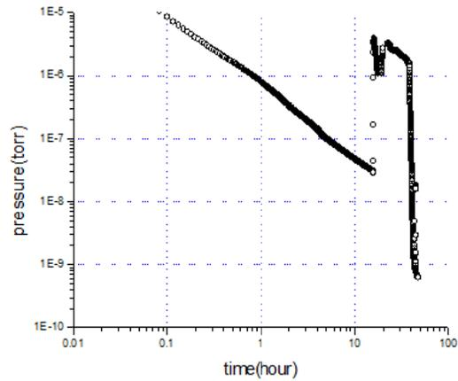
Figure 5: Pumping curve for the OFHC absorber.
