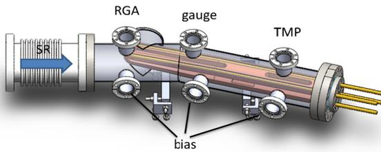
Figure 4: PSD system of the crotch absorber
