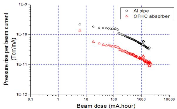
Figure 6: Total pressure rise per beam current as a function of beam dose for OFHC and Al absorbers
