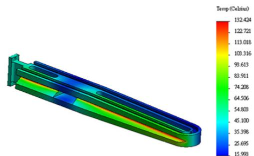
Figure 2: Temperature distribution of the crotch absorber.
