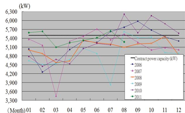
Figure 2: Monthly peak power consumption in NSRRC from 2006 to 2011.
