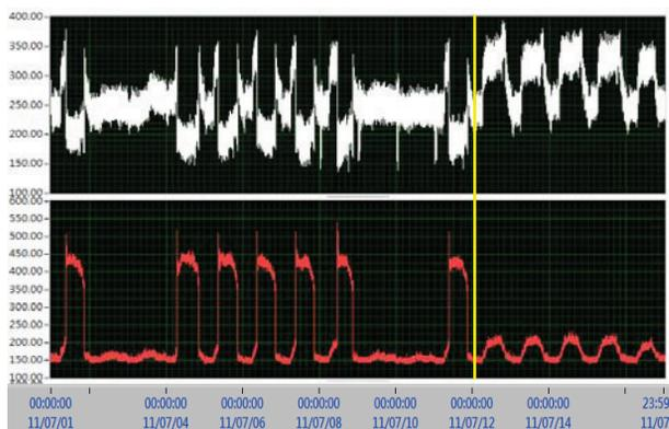
Figure 3: Power consumption of ID building before and after the chiller operation control change.
