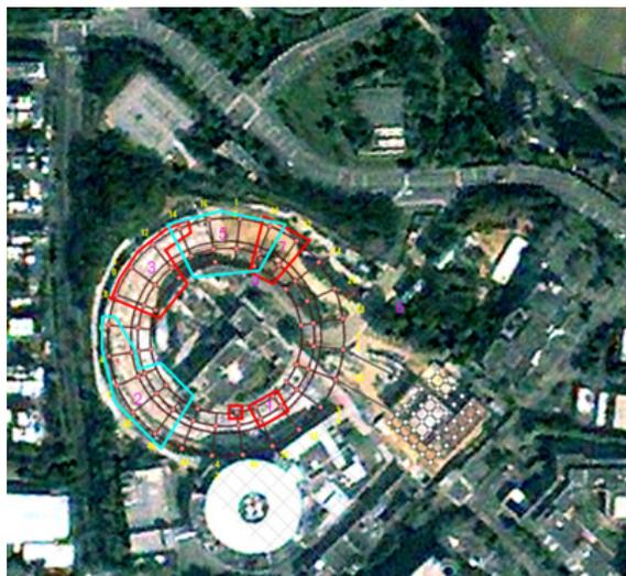
Figure 1: The TPS construction site and the layout of the ground grid. The blocks and numbers in the graph indicate the order of ground resistance measured, Table 1.
