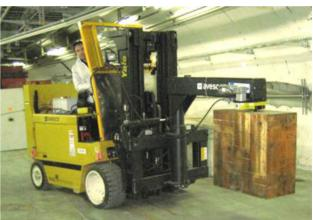
Figure 2: Shielded Forklift equipped with automatic hook.
