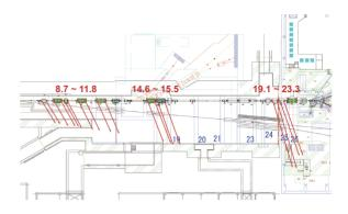
Figure 8: Horizontal displacements of hadron beam line.
