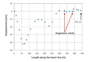
Figure 1: Subsidence of LINAC. Start point is used as the base.
