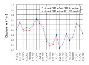
Figure 2: Subsidence of RCS. RCS\_01 is used as the base.
