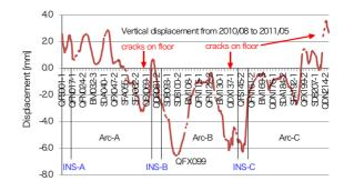
Figure 4: Subsidence of main ring. Level zero is arbitrary.
