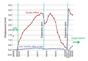
Figure 7: Subsidence of neutino beam line. MHR38 is used as the base.
