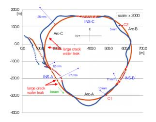
Figure 5: Horizontal displacements of 3-50BT line and main ring.
