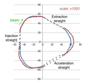
Figure 3: Horizontal displacements of RCS.
