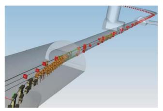
Figure 1: 3D visualization of the area of positron injection into the damping ring complex of the ILC. Several models have been combined for this figure: 3D CAD models of the positron source accelerator components and of the tunnel facilities, and a schematic illustration of the damping ring lattice.
