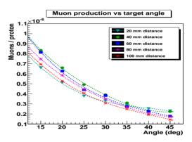
Figure 4: Muon production as a function of target angle for a set of two slabs.
