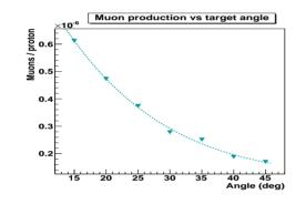
Figure 2: Muon production as a function of the target angle for the original ISIS target.
