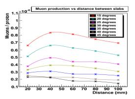
Figure 5: Muons production as a function of slabs distance.
