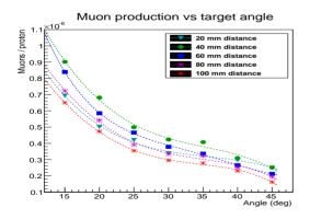
Figure 7: Muon production as a function of target angle for a set of three slabs.
