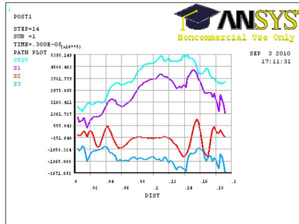
Figure 3: Equivalent stress (σ<sub>eq</sub>), and its components (σ<sub>1</sub>, σ<sub>2</sub>, σ<sub>3</sub>) along the path of the beam in the beryllium spoiler 3 μs after a bunch train hit. The main contributor to the stress is σ<sub>1</sub> and it is of tensile nature.
