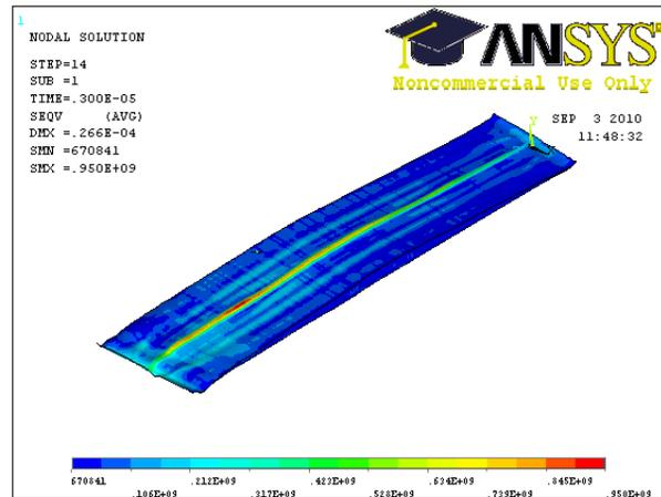
Figure 2: Equivalent stress in the beryllium spoiler 3 μs after the bunch train hit.
