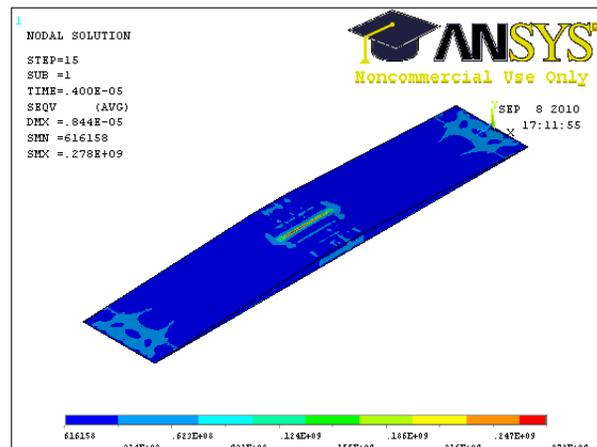
Figure 4: Equivalent stress in the beryllium spoiler 4 μs after the bunch train hit.
