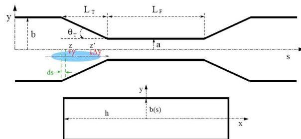
Figure 1: Longitudinal view of a tapered collimator. An oncoming particle bunch is schematically represented by the solid ellipse. Not to scale.
