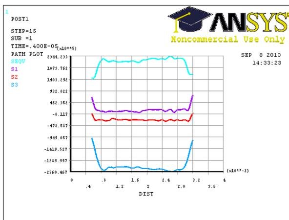
Figure 5: Equivalent stress ( $\sigma_{eq}$ ), and its components ( $\sigma_1$ ,  $\sigma_2$ ,  $\sigma_3$ ) along the path of the beam in the beryllium spoiler 4  $\mu$ s after a bunch train hit. The main contributor to the stress is  $\sigma_3$  and it is of compressive nature.
