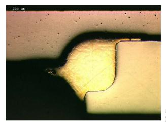
Figure 2: Micrograph of a Be-Stainless steel vacuum brazed joint.
