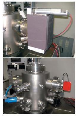
Figure 3: Picture of the UHV test bench with the SIP and the NEXTorr® D100-5 installed.
