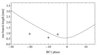
Figure 4: Preliminary ALICE bunch length measurements as a function of BC1 phase (crosses) and ASTRA simulation (line). The bunch charge is 60 pC and the buncher power is 0.53 kW.
