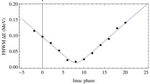
Figure 5: ALICE post-linac energy spread vs linac phase. The points are measurements, the line is a fit of Equation (1) where the free parameters are bunch length and minimum energy spread. A bunch length of 1.3 mm FWHM is extracted.
