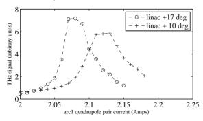
Figure 6: ALICE THz signal vs first arc quadrupole strength, for two fixed linac off-crest phases. Two quadrupoles (symmetrically positioned about the central arc dipole) are varied together to vary the post-linac  $R_{56}$ .
