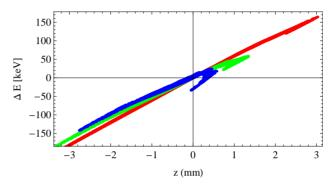
Figure 3: ALICE simulated injector longitudinal phase space as a function of BC1 phases. BC1=-20° (red), -10° (green), -5° (blue).
