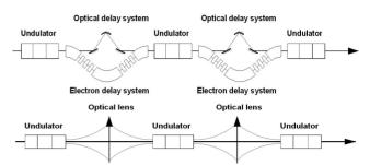
Figure 1: Scheme of the installation and its equivalent optical analog.
