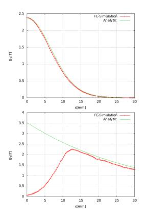
Figure 7: Comparison of By(x) for FE-simulations and analytic field models.
