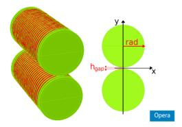
Figure 3: Schematic view of the cylindrical undulator.
