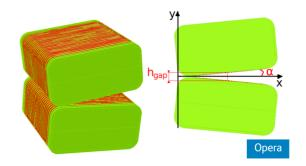
Figure 4: Schematic view of the tilted undulator.
