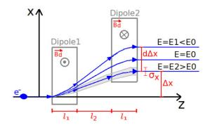
Figure 2: Schematic view of the chicane.
