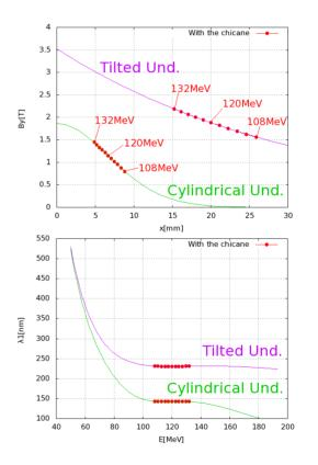
Figure 5: Comparison of calculated and required flux densities and resulting wavelengths for both geometries.
