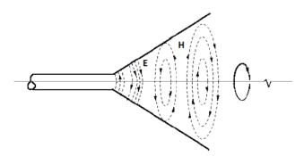
Figure 4: Conical coaxial launcher for generating a surface travelling wave to simulate an electron beam.
