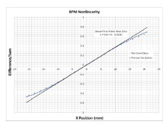
Figure 2: Plot of the nonlinearity of a BPM in the rotated X mid-plane. Linearity holds to about 8 mm from center.
