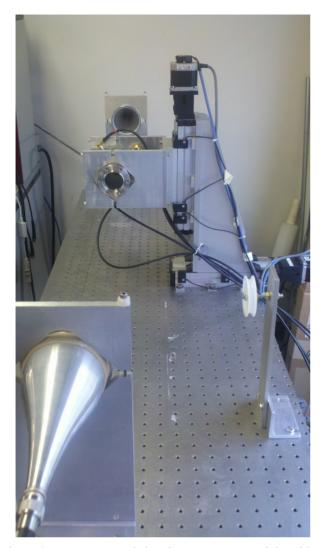
Figure 3: BPM test stand showing X-Y stage at right with a mounted BPM. The 160 micron wire stretched between the RF cones at both ends of the system simulates a beam.
