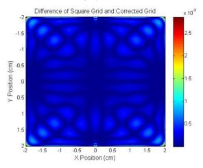
Figure 9: Colour map showing the precision of the polynomial correction for the X-plane. The Y-plane has similar results.
