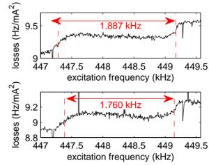
Figure 2: Normalised loss rate vs. excitation frequency for cavity voltages of 2.6 MV (top) and 2.4 MV (bottom).
