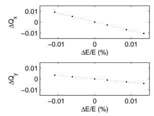
Figure 5: Horizontal (top) and vertical (bottom) tune shift as a function of relative change in beam energy. The slope of the data gives the measured natural chromaticity.
