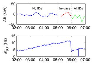
Figure 3: Measured beam energy over a 5 hour period with and without ID changes (top). RF frequency during the measurements (bottom).
