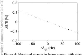
Figure 4: Measured change in beam energy with change in RF frequency. The slope of the curve can be used to calculate the momentum compaction factor.
