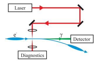
Figure 1: Schematic layout of the laser-wire.
