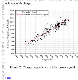
Figure 2: Charge dependence of Cherenkov signal.
