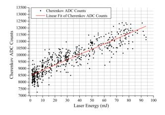
Figure 3: Laser energy dependence of Cherenkov signal.
