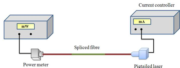
Figure 5: Schematic of the experimental setup used for testing the second arm of the sensor.
