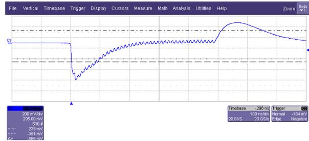
Figure 4: Detector response for 50 bunches with a spacing of 12 ns.
