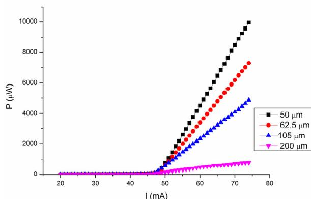
Figure 6: Measured power versus laser current with different spliced fibres. The black squares show the reference line (50  $\mu\text{m}$  core, without any splicing).
