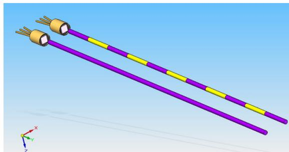
Figure 1: Schematic showing two arms of the optical fibre beam loss monitor.
