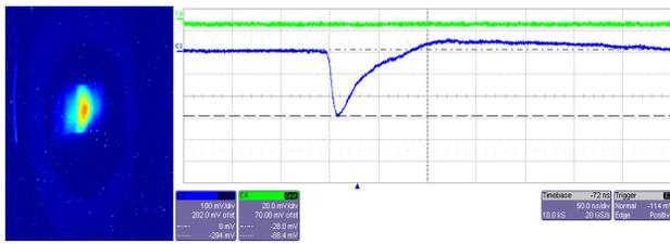
Figure 2: Left: transverse profile of a beam in ALICE with energy 27.5 MeV and bunch charge 63 pC. Right: Detector response (blue line) when the beam is passing through the fibre.
