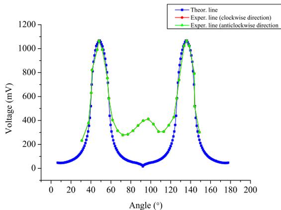
Figure 3: Maximization of the Cherenkov angle as a function of the signal amplitude in both directions compared with the theoretical curve (blue squared line).
