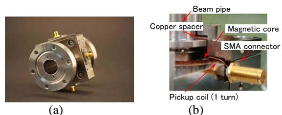
Figure 1: (a) Photograph of a high-speed differential CT monitor and (b) the inner structure.
