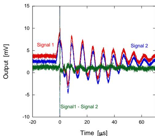
Figure 2: Output signals of the differential CT with environmental noise. The signal 1 (red line) and signal 2 (blue line) are raw data from the CT. The signal 1 is positive output and the signal 2 is negative one. The green line is a subtracted signal from signal 1 to signal 2.
