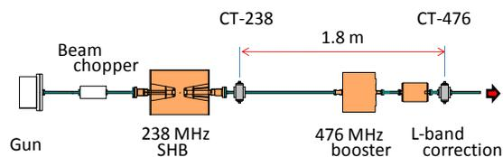
Figure 4: Layout of the injector part in the SACLA.
