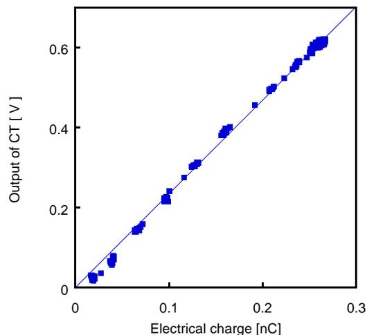
Figure 3: Output response of the CT versus the electron charge for the electron beam of the SCSS test.
