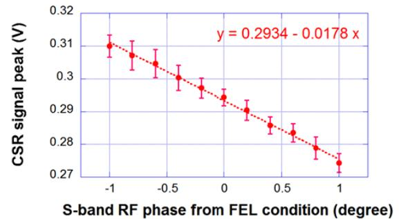
Figure 6: Rf phase dependence of CSR intensity at BC2.
