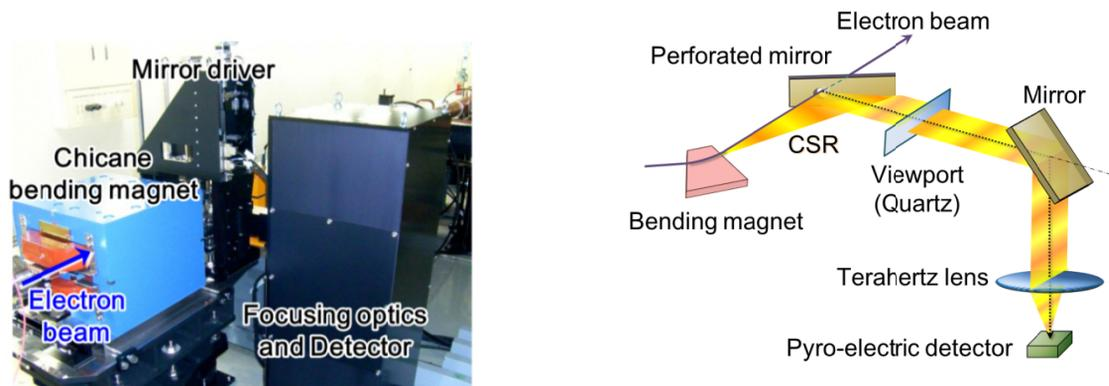
Figure 2: (Left) Set-up of the CSR monitor instruments at the BC2, and (Right) their schematic layout. The focusing optical system and detector are installed in the black case to reduce an unnecessary light from the exterior.
