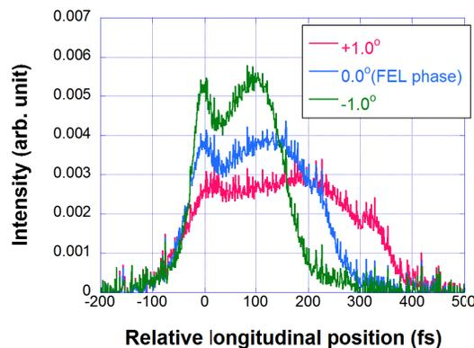
Figure 5: Longitudinal distribution of beam at the exit of BC2 measured by the rf deflector cavity. The index phases indicate the rf phase of S-band accelerators.
