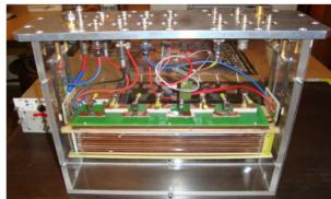
Figure 2: First GEM-TPC prototype assembled in laboratory.
