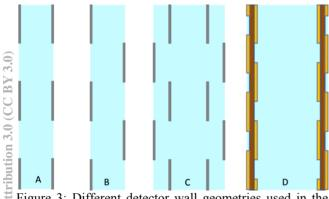
Figure 3: Different detector wall geometries used in the simulations. The dimensions of the elements are not in scale. A represents the configuration used in the prototype GEM-TPC, B with interlocked strips, C with double strips and D with strips etched on copper coated Kapton foil.
