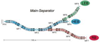
Figure 1: Layout of the Main-Separator of the Super-FRS. The detection systems will be placed on front and back of each focal point marked as MF with numbering from 1 to 9. Low energy branch has three more focal points outside the area of this layout.
