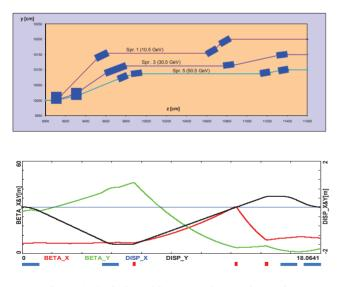
Figure 3: Switchyard layout and spreader optics.
