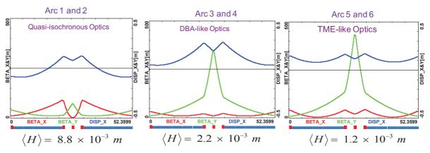
Figure 4: Various flavours of FMC Optics used for different energy arcs with appropriate values of <H>.
