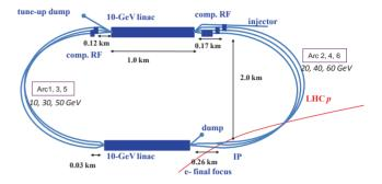
Figure 1: Schematic layout of a 3-pass up/3-pass down ERL.
