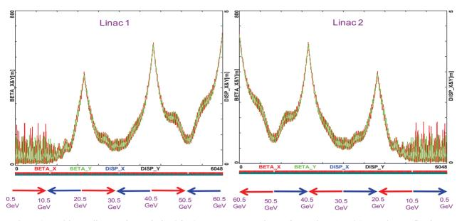
Figure 2: Multi-pass linac optics optimized for 3-pass ERL As a virtue of ER, Linac 1 and 2 are mirror reflections.
