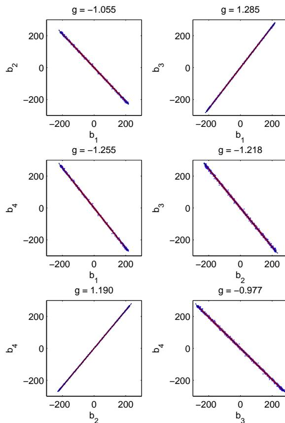
Figure 3: Calibration data from one BPM at CsrTA. Each plot shows the correlation between button signals for 1024 turns of an electron bunch, during resonant excitation in normal mode I. The blue points show the data; the red lines show ellipses fitted to the data. The gradient of the major axis of the ellipse (given as the value  $g$  above each plot) gives a component of the calibration matrix  $B$ .
