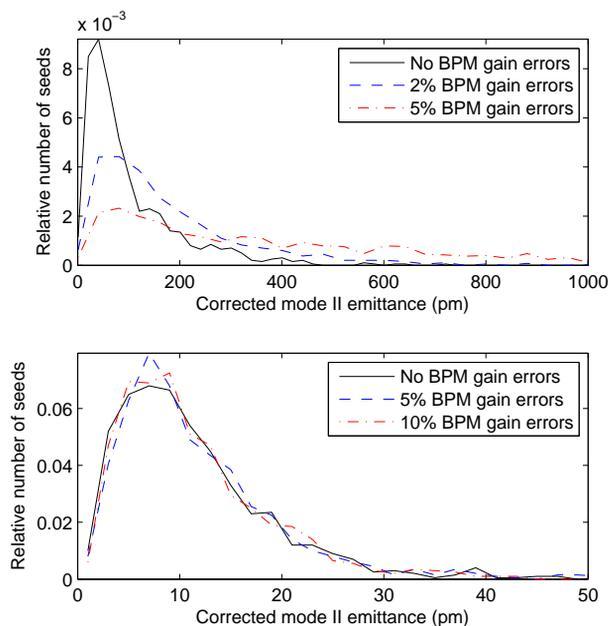
Figure 2: Simulations of emittance correction in CsrTA. Top: distribution of final mode II emittance after orbit and vertical dispersion correction. Bottom: as the top plot, but with correction based on mode II dispersion, rather than vertical dispersion. 1000 seeds of machine error are simulated.
