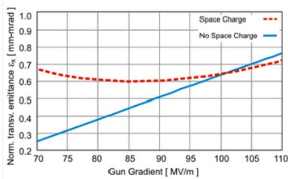
Figure 2: Transverse emittance at the gun exit versus the acceleration gradient in RF cavity. The results with (red) and without (blue) space charge effects are shown.
