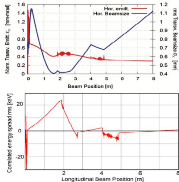
Figure 7: Transverse normalized emittance, beamsize (top) and correlated energy spread (bottom) evolution along the linac.
