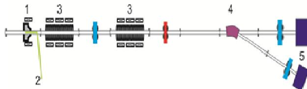
Figure 1: Schematic layout of AREAL 20 MeV S-Band linear accelerator. 1- RF -photo gun, 2- laser, 3- S-Band accel. sections, 4 –spectrometer, 5 - Beam dump.
