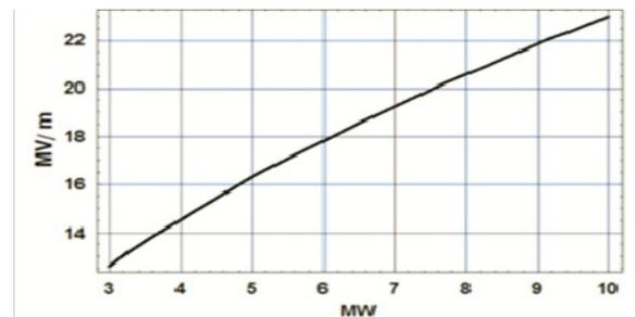
Figure 5: Obtained gradient vs RF power for S-Band accelerating sections.
