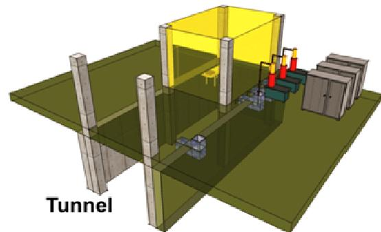
Figure 2: The AREAL tunnel and supply infrastructure.
