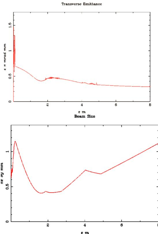
Figure 6: Transverse normalized emittance (top) and beam rms size (bottom) evolution along the linac.
