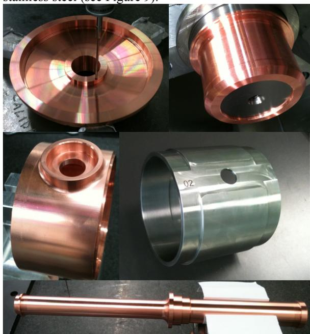
Figure 9: Different parts of the drift tubes for Linac4.
