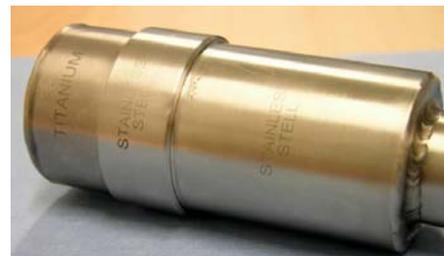
Figure 5. The world first sample of Ti-SS bimetallic transition element prepared to the leak tests in INFN.
