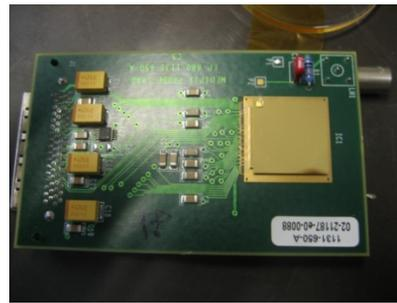
Figure 2: Spectrometric detector based on GaAs (Cr) pixel sensor with 256x256 channels of 50  $\mu\text{m}$  resolution and Medipix chip.
