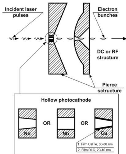
Figure 4: Scheme of the hollow photocathode.
