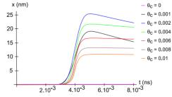
Figure 5: Horizontal deviation of the central trajectory with respect to the machine axis during collision for ILC nominal beam parameters.
