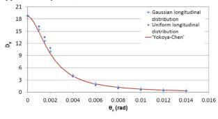
Figure 3: Vertical disruption parameter as a function of  $\theta_c$  for ILC nominal beam parameters.
