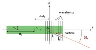
Figure 2: Schematic of the electromagnetic interaction.
