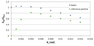
Figure 4: Beamstrahlung parameter as a function of  $\theta_c$  for ILC nominal beam parameters,  $\delta_{BS,n} = 2.1\%$ .
