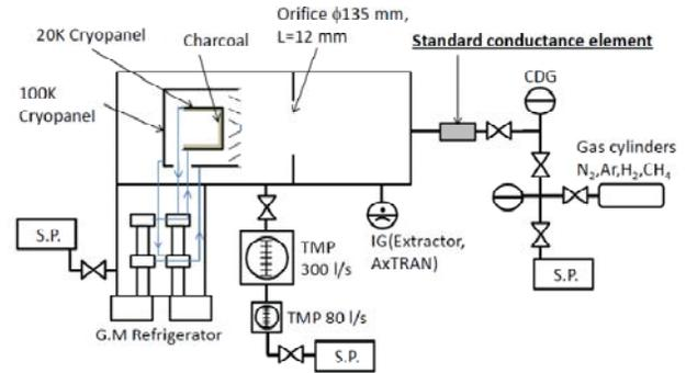
Figure 3: A 20 K bakeable cryopump and a pump speed measurement system with a precise gas flow control system using a standard conductance element.
