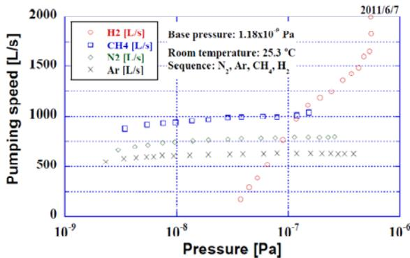
Figure 4: Result of the pumping speed of the 20 K bakeable cryopump for hydrogen, methane, nitrogen and argon.
