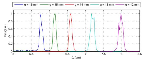
Figure 3: ALICE FEL spectra at different undulator gaps.
