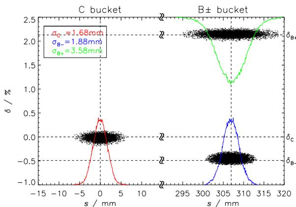
Figure 5: MAD-X simulation of an asymmetric triple beam stored at the MLS,  $(\alpha_0, \alpha_1, \alpha_2) = (-0.00145, -0.23, 14)$ ,  $E_0 = 629 \text{ MeV}$ ,  $U_0 = 250 \text{ kV}$ .
