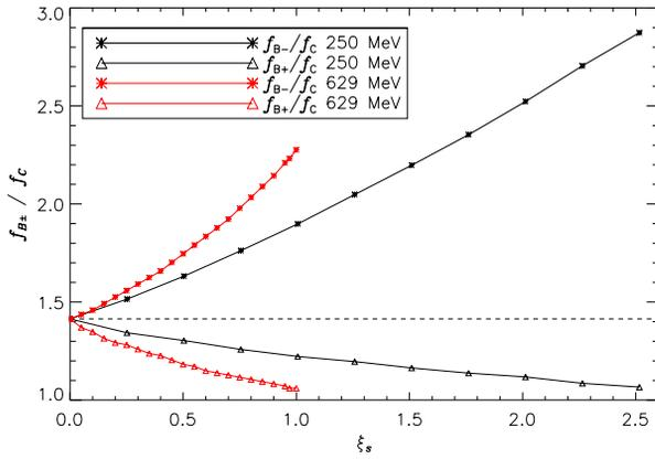
Figure 4: Measured longitudinal synchrotron oscillation frequencies of the buckets  $B_{\pm}$  while varying  $\xi_s$ .
