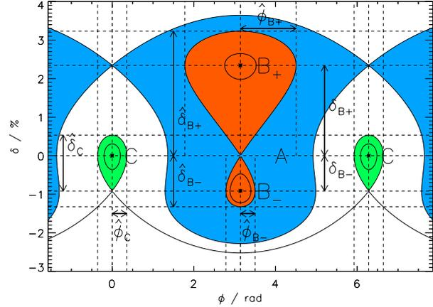
Figure 1: Longitudinal phase space featuring alpha buckets dominated by  $\alpha_2$  ( $\alpha_0, \alpha_1 < 0$ ;  $\alpha_2 > 0$ ) and characteristic parameters (see text).
