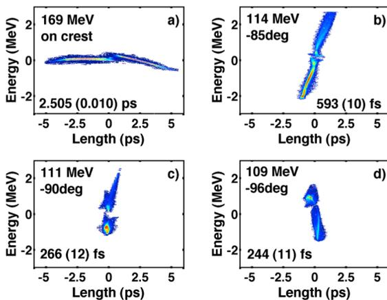
Figure 4: Measured LPS for a two pulses comb beam; the label reports the average energy, the compression phase and the rms bunch length (150 pC in each sub-bunch).
