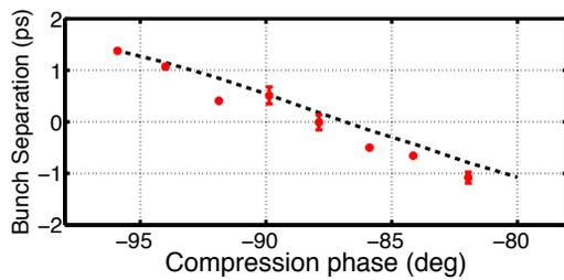
Figure 3: Measured bunch separation for a two bunches train compared to TSTEP simulation (total charge 160 pC).
