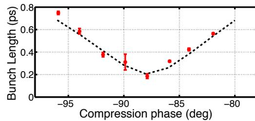
Figure 2: Measured compression curve for a two bunches train compared to TSTEP simulation (total charge 160pC).
