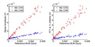
Figure 6: Scraping at TCP.D6L7 vertical collimator. BLM vs. microphone signal (left) and vs. FFT component at  $f_{rev}$  (right). A linear dependency can be seen for both effects. Microphone CH6 is more sensitive to losses than CH5.
