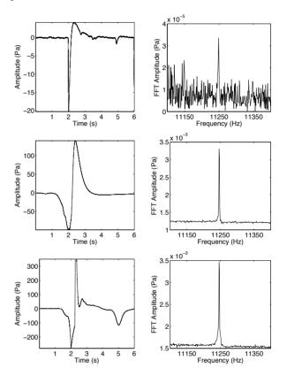
Figure 4: Spikes in microphone signals during beam losses with low, medium and high loss rates (top, middle, bottom). Amplitude vs. time (left) and FFT Amplitude vs. frequency (right). FFT size of 200 ksamples, 1s window triggered at the beginning of the spike, Hanning window.
