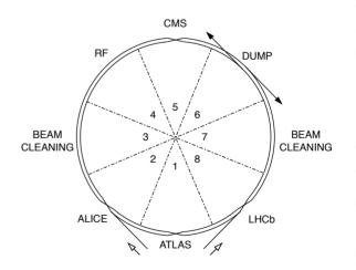
Figure 1: Scheme of the eight LHC sections. Microphones have been installed at all primary collimation regions in sector 3 and 7 for both beams.
