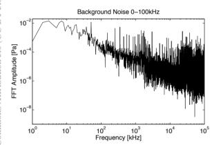
Figure 3: FFT of background noise in IP7 left. Tonal components are mainly EM induced noise.
