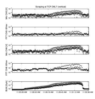
Figure 5: Comparison of microphone signals CH5 and CH6 with a running sum of 1.3 s and a sample rate of 1Hz, the corresponding FFT bins at  $f_{rev}$ , and the reference BLM signal at collimator TCP.C6L7 during a scraping at TCP.D6L7 vertical collimator. A similar response to losses can be seen in all signals. Loss spikes exceed background noise level at approximately  $10^{-4}$  Gy/s for both microphones.
