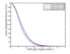
Figure 4: Normalized integrated lost beam intensity versus jaw postion in units of measured beam sigma, during vertical (purple), horizontal (blue) and skew (black) scrapings on B2.
