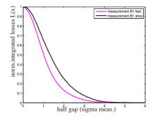
Figure 5: Comparison of normalized integrated lost beam intensity,  $I_{tot,lost}(u)/I_{total}$ , versus jaw position in units of measured beam sigma,  $\sigma_{meas}$ , during slow (black) and fast (purple) vertical scraping on B1. Note: It was assumed  $\sigma_{meas} = 0$  for the collimator jaw position  $u_i = \mu_{i,0}$ , with the fitted beam offset  $\mu_{i,0}$  for scraping *i*.
