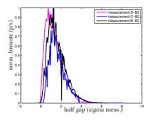
Figure 2: Normalized instantaneous loss rates during the scraping experiments on B2 versus the collimator half gap in units of measured beam size,  $\sigma_{meas}$ . The scrapings were performed in the vertical (purple), horizontal (blue) and skew plane (black) with the respective primary collimators in IR7: D-ver, C-hor and B-skew.
