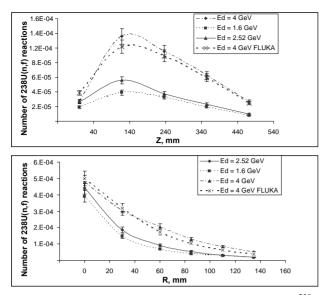
Figure 2. Spatial distributions of fission reactions  $^{238}$ U (n,f) at deuteron energies of 1.6, 2.52, 4 GeV. Data are given per  $^{238}$ U gram and one deuteron incident on the target: top picture shows axial distributions (R = 85, along the axis of the blanket), bottom picture gives radial distributions (Z =118).
