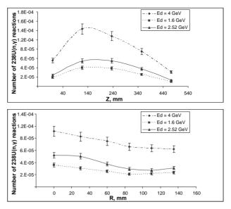
Figure 1. Spatial distributions of neutron capture reactions  $^{238}$ U(n, $\gamma$ ) at deuteron energies of 1.6, 2.52, and 4 GeV. The data are given for one  $^{238}$ U gram and one deuteron incident on the target: top picture shows axial distributions (R = 60, along the axis of the blanket), bottom picture gives radial distributions (Z = 118).
