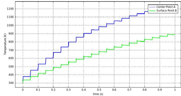
Figure 1: Temperature evolution in the central point (A in blue) and a point on the surface (B in green) during the first second of irradiation (20 pulses).
