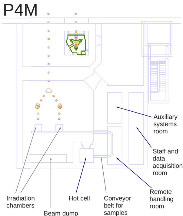
Figure 3: Basic layout of the P4M laboratory.
