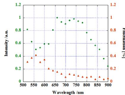
Figure 4: The intensity spectra (●) and stability (▲) of SC generated from the single laser
