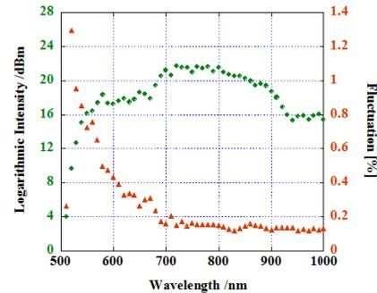
Figure 3: The intensity spectra (●) and stability (▲) of SC generated from the 119 MHz laser
