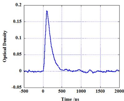
Figure 6: The transient absorption decay of water sample at 800 nm
