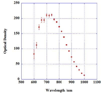
Figure 7: The absorption spectra of hydrated electron
