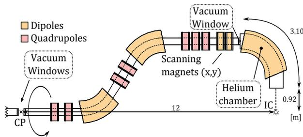
Figure 1: Schematics of one proton gantry option: double CP vacuum windows and helium in last bending dipole. Without helium in the dipole, the last vacuum window would be located just before the nozzle.
