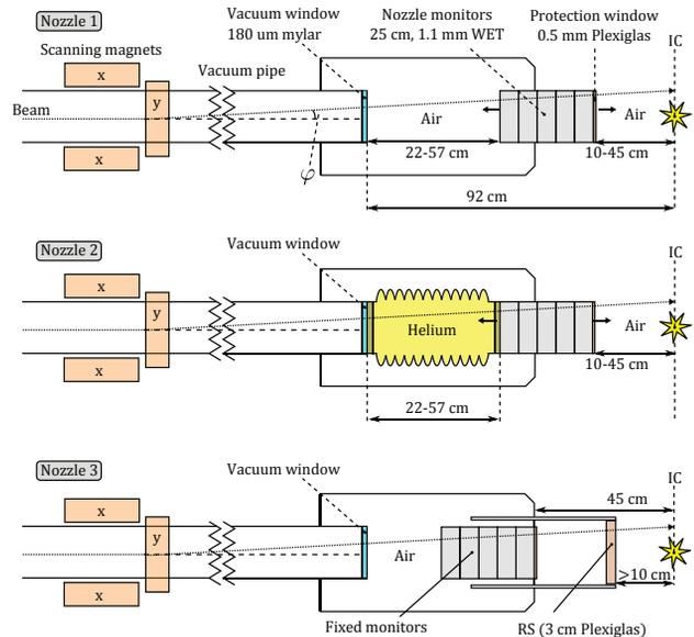
Figure 2: Different nozzle options. 1: Movable monitors. 2: Movable monitors and helium chamber after vacuum window. 3: Fixed monitors, movable (and removable) range shifter.
