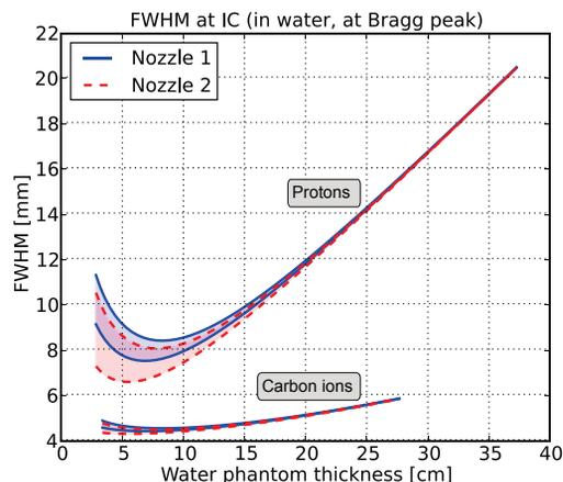
Figure 4: FWHM at IC, in water (at Bragg peak). Upper bands: 60-250 MeV protons, lower bands: 120-400 MeV/carbon ions.
