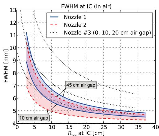
Figure 3: FWHM (horizontal and vertical) in air vs. residual beam range in water,  $R_{res}$ , at the IC. The three dotted lines indicate IC beam sizes for Nozzle 3, assuming 0, 10 and 20 cm air gap between RS and IC.
