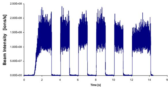
Figure 4: Five arbitrary spill pauses are applied to a carbon beam.
