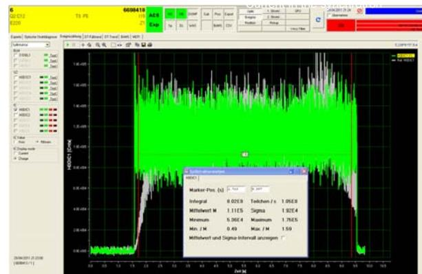
Figure 3: Spill shape for carbon beam with (green) and without (grey) feed back.
