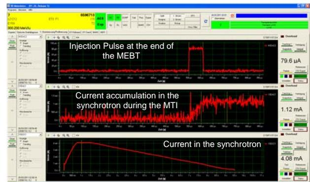
Figure 2: Standard synchrotron cycle for carbon ions of an energy of about 300 MeV/u.
