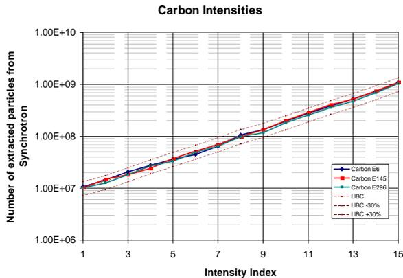
Figure 1: Number of extracted carbon ions per spill for different intensities.
